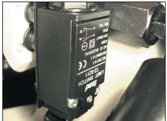
Figure 61. G0613 blade stop limit switch.
